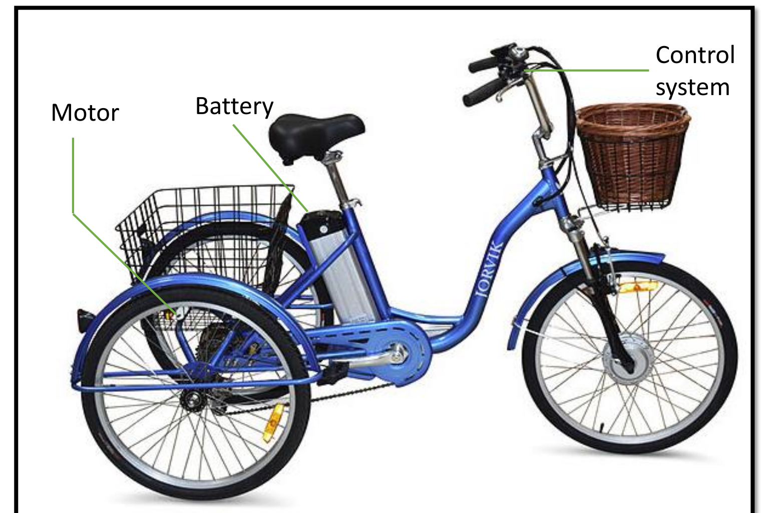
Figure 1: The e-trike and its components
